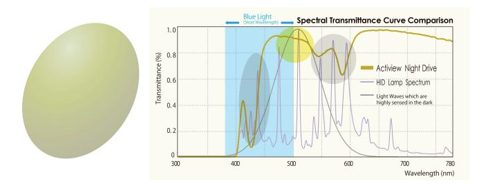
The medical filter has a dimming effect on glaring light without darkening the overall view. It also increases the contrast, resulting in clearer vision.
